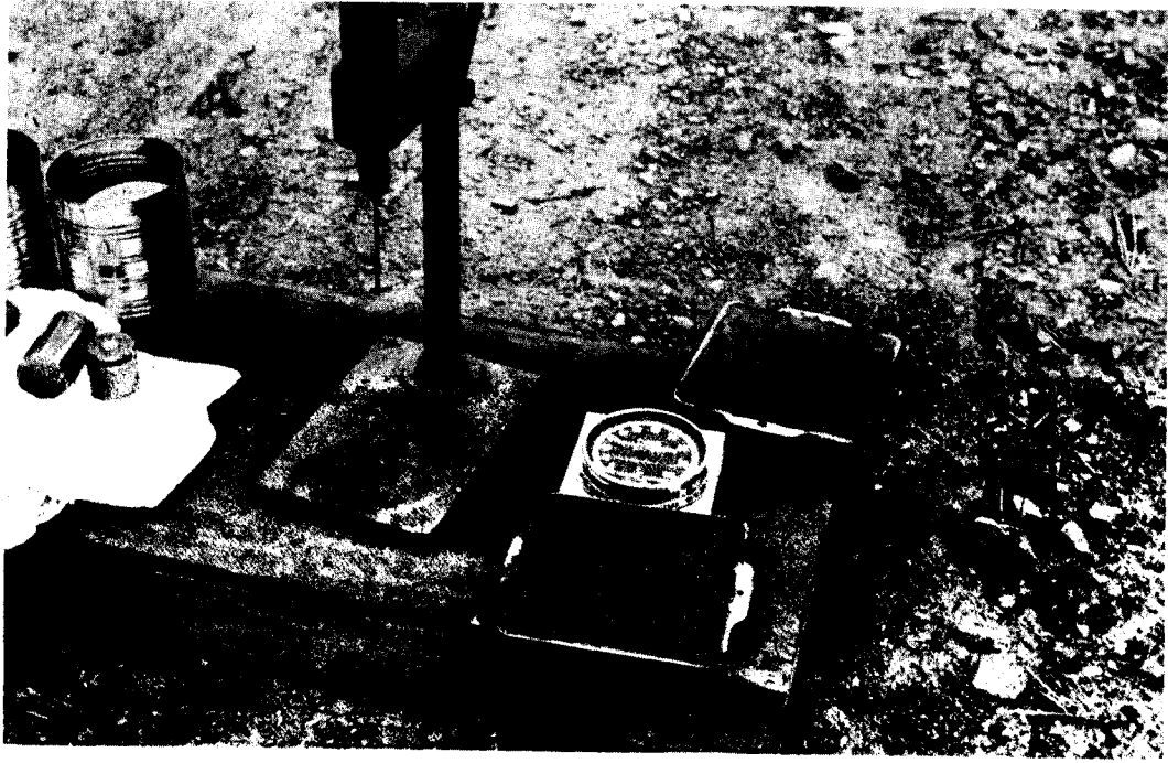
Figure 13. View of specimens used in measurement of moisture loss. Also shown are the instrument for measuring relative humidity and the penetrometer used in ASTM C 403.
