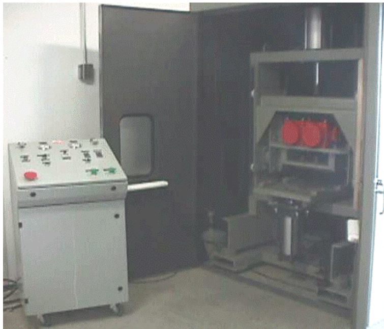
Figure 1. PTI Vibratory compactor.
