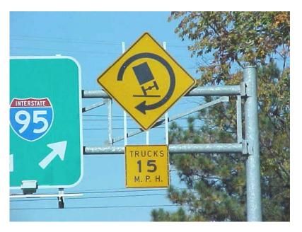
Figure 2. Static Truck Rollover Sign
