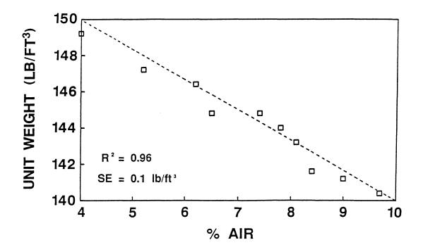
Figure 3. Relationship between the air content measured by a Type A pressure meter and the unit weight of the fresh concrete.
