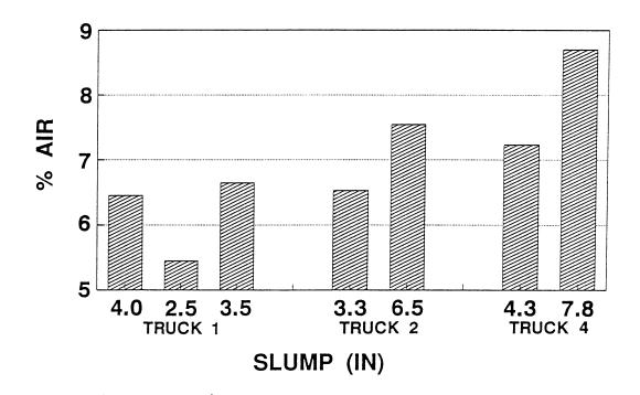
Figure 6. Air content and slump after the addition of water.
