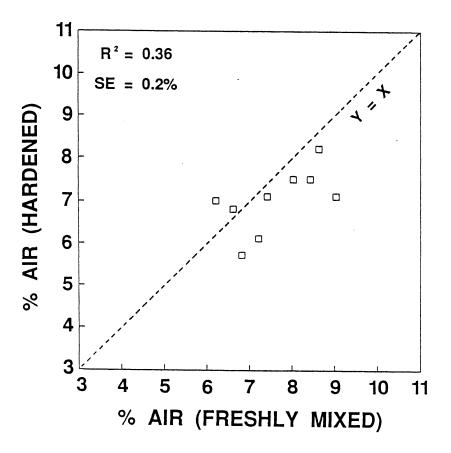
Figure 7. Comparison of air content of concretes from Plant 2 determined with a Type A pressure meter in the fresh stage with that determined microscopically in the hardened stage.
