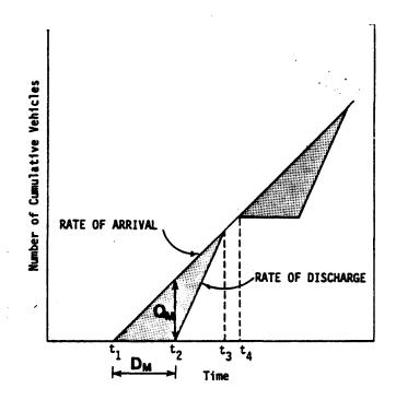
Figure 9. Volume/capacity relationship when traffic stream is temporarily stopped. (From reference 6.)
