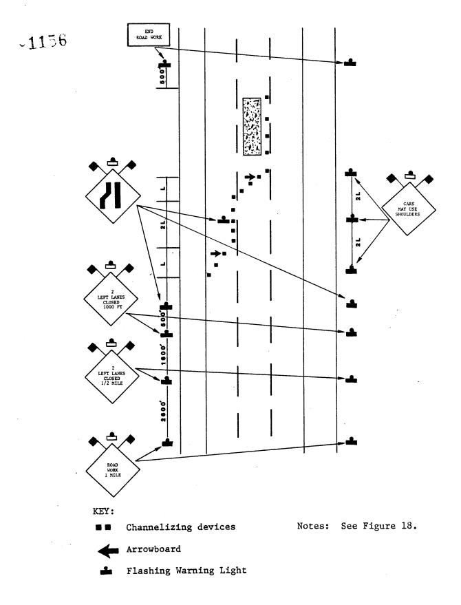
Figure 20. Typical layout for use of shoulders.
