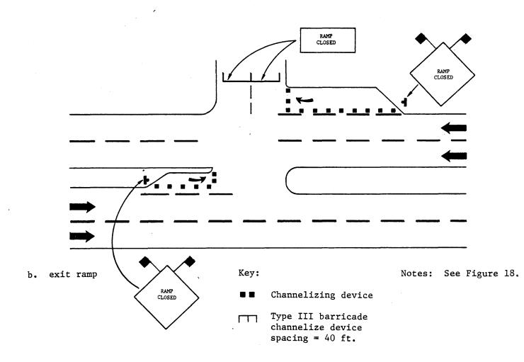
Figure 23. Typical layouts for ramp closures.
