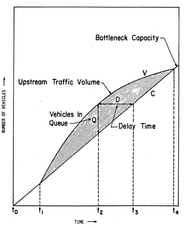
Figure 6. Traffic volume-capacity relationships when queuing occurs. (From reference 8.)
