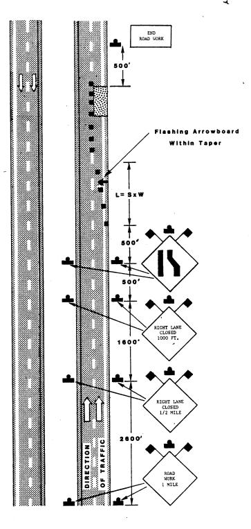
Figure 17. Typical layout for a single-lane closure.
