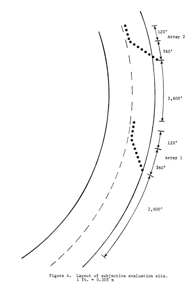
There was a slight horizontal curve and upgrade prior to the first taper and a slight curve and downgrade prior to the second one. Some observers noted that the second taper was more visible than the first due to the geometrics and the background. However, the data did not indicate that the road geometrics were a significant influence.
