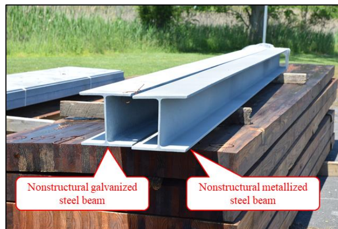
Figure 13. Photograph of Nonstructural Galvanized and Metallized/Sealed Steel Beam at the 2022 Holdens Creek Bridge Site Prior to Installation
