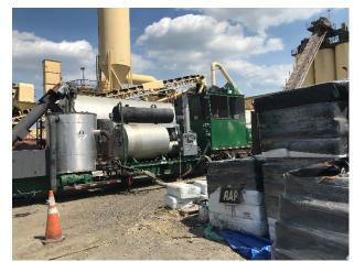
Figure 6. GTR and Asphalt Binder Mixing Tank to the Left and System Control House to the Right. GTR = ground tire rubber.
