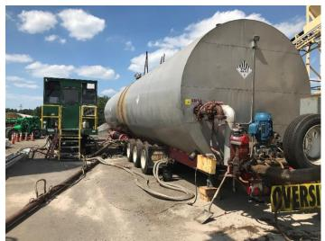
Figure 7. Asphalt Rubber Binder Holding Tank
