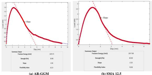
Figure 11. Example Load Displacement Plot From SCB Test. SCB = semi-circular bend test
