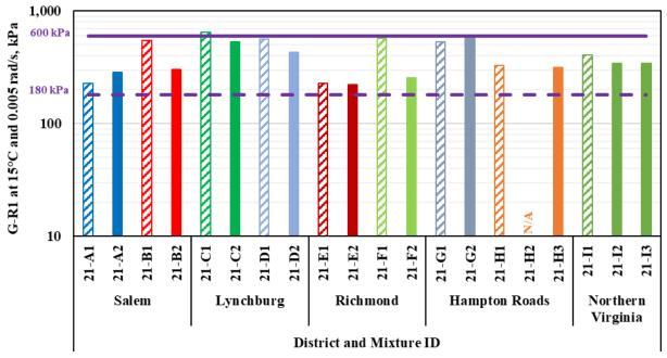
Figure 13. Glover-Rowe (G-R1) Values at 15°C and 0.005 rad/s of the Evaluated Binders at 20-Hour PAV Aging Conditions. Purple dashed and solid lines indicate onset and significant cracking limits, respectively. PAV = pressure aging vessel; N/A = not available.
