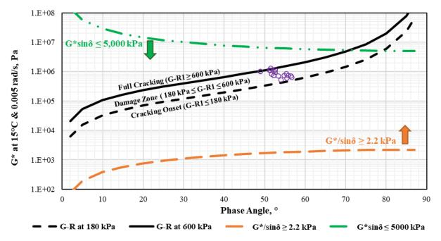
Figure 14. Black Space Diagram in Terms of Glover-Rowe (G-R1) Values at 15°C and 0.005 rad/s for 2021 Binders at 20-Hour PAV Aging Conditions. PAV = pressure aging vessel;  $G^* = \text{complex shear modulus}$ ;  $\delta = \text{phase angle}$ .
