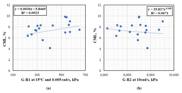
Figure 22. Correlation Between CML and (a) G-R1 at 15°C and 0.005 rad/s and (b) G-R2 at 10 rad/s. CML = Cantabro mass loss; G-R = Glover Rowe parameter.
