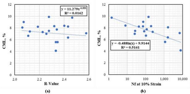
Figure 23. Correlation Between CML and (a) R-Value and (b) LAS Binder Fatigue Parameter, N<sub>f</sub>, at 10% strain. CML = Cantabro mass loss; LAS = linear amplitude sweep.
