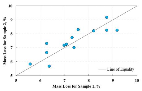
Figure 9. Within-Lot Sample-to-Sample Comparison for Cantabro Test
