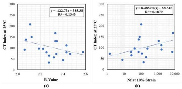
Figure 21. Correlation Between CT Index and (a) R-Value and (b) LAS Binder Fatigue Parameter, N<sub>f</sub>, at 10% strain. CT = cracking tolerance; LAS = linear amplitude sweep.
