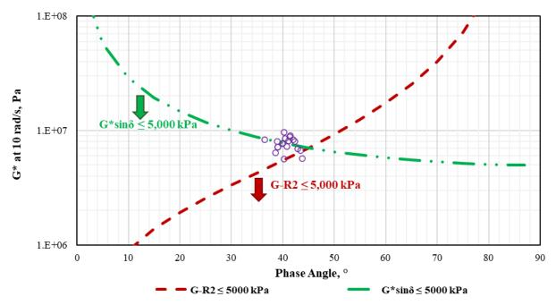
Figure 16. Black Space Diagram in Terms of Glover-Rowe (G-R2) Values at the Corresponding Binder Fatigue Test Temperature and 10 rad/s of the Evaluated Binders at the 20-Hour PAV Aging Conditions. PAV = pressure aging vessel;  $G^*$  = complex shear modulus;  $\delta$  = phase angle.
