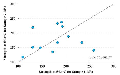
Figure 12. Within-Lot Sample-to-Sample Comparison for Indirect Tensile Test at High Temperature
