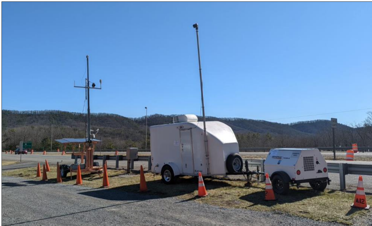
Figure 16. APRS Trailer and Supporting Equipment Installed Adjacent to the Northbound Outer Lane of I-77 Near the Walker Mountain Tunnel
