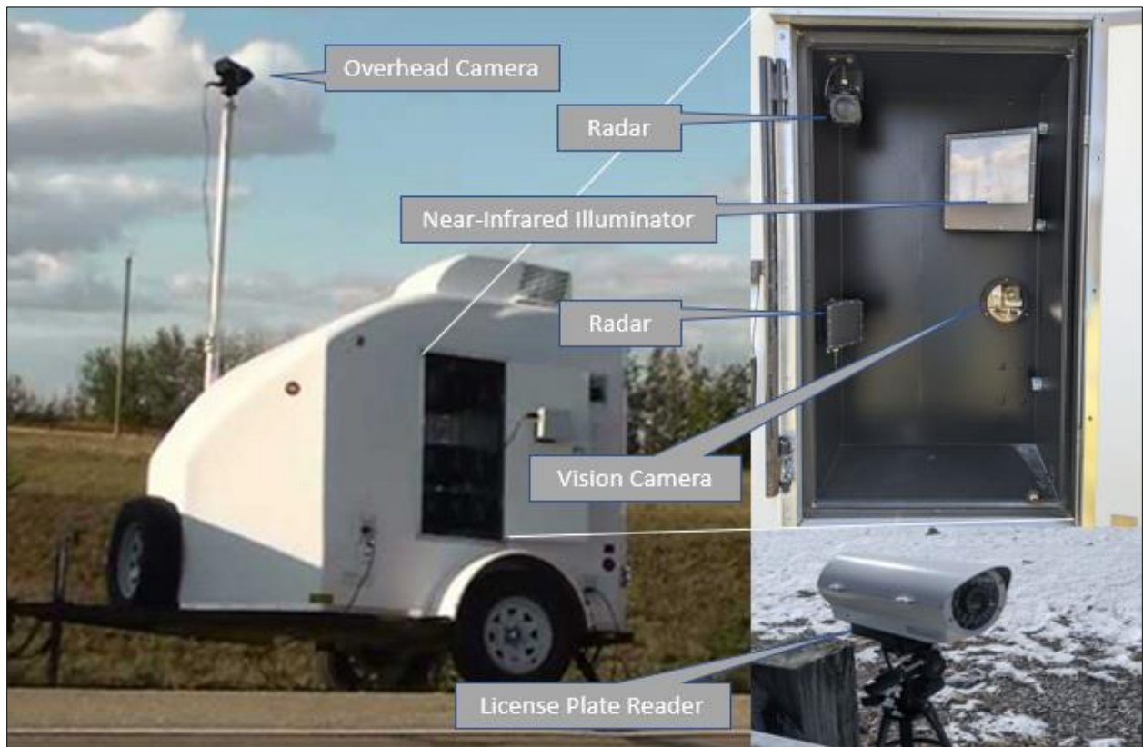
Figure 1. Mobile Automated Placard Reader System (APRS) Trailer with System Component Types and Locations Shown
