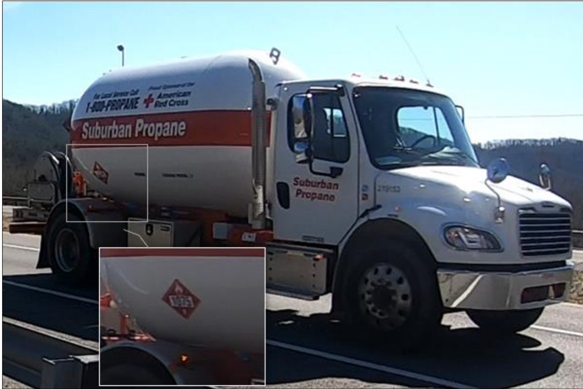
Figure 23. Example of a False Negative, Still Image from Captured Footage Showing the Placard Clearly Visible, Likely Meaning a True False Negative
