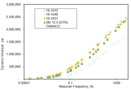
Figure 8. Dynamic Modulus Results (Semi-log Scale). Mixtures 18-1012, 18-1946, and 18-1057 are conventionally modified SM-12.5E mixtures from the previous season in the same district. GTR = ground tire rubber; THMACO = thin hot mix asphalt concrete overlay.
