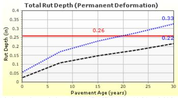
Figure C1. Rutting Prediction Using Existing Rutting Coefficients:  $k1*\beta1 = -2.304$ ;  $k2*\beta2 = 1.5606$ ;  $k3*\beta3 = 0.4791$ .
