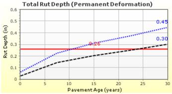
Figure C2. Rutting Prediction Using Different Rutting Coefficients:  $k1*\beta1 = -3.35412$ ;  $k2*\beta2 = 1.5606$ ;  $k3*\beta3 = 0.4791$ .
