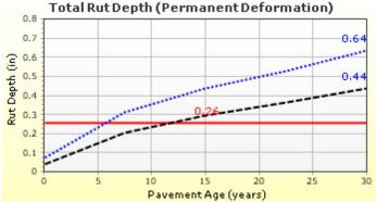
Figure C3. Rutting Prediction Using Different Rutting Coefficients:  $k1*\beta1 = -5.03118$ ;  $k2*\beta2 = 1.5606$ ;  $k3*\beta3 = 0.4791$ .
