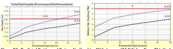
Figure B5. Predicted Rutting and Bottom-Up Cracking With Average SM-E Values From This Study and Existing Values for IM and BM. SM-E = dense-graded polymer modified; IM = intermediate mix; BM = base mix.
