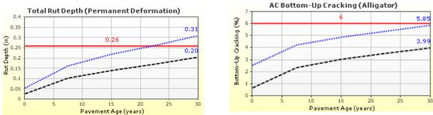
Figure B4. Predicted Rutting and Bottom-Up Cracking (With SM-E Values for Mix 18-1011 and Existing Values for IM and BM). IM = intermediate mix; BM = base mix.
