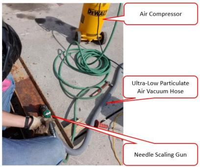
Figure 4. Pneumatic Needle Scaler Configuration
