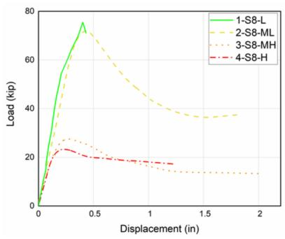
Figure 28. Load vs. Displacement Data for S8x18.4 Beams
