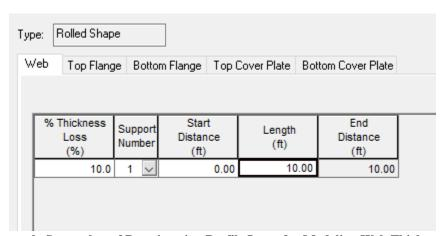
Figure 22. Example Screenshot of Deterioration Profile Input for Modeling Web Thickness Loss in BrR
