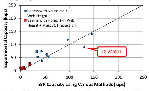
Figure 51. Comparison of Experimental and BrR Capacity Using Various Methods for Effective Web Thickness
