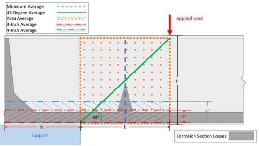
Figure 21. Methods for Calculating Average Web Thickness
