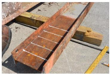
Figure 14. Specimen 1-S8-L Stripped of Paint
