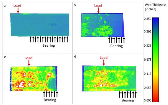
Figure 24. Heat Maps Showing Web Thickness of S8x18.4 Beam End Specimens: (a) 1-S8-L; (b) 2-S8-ML; (c) 3-S8-MH; (d) 4-S8-H.
