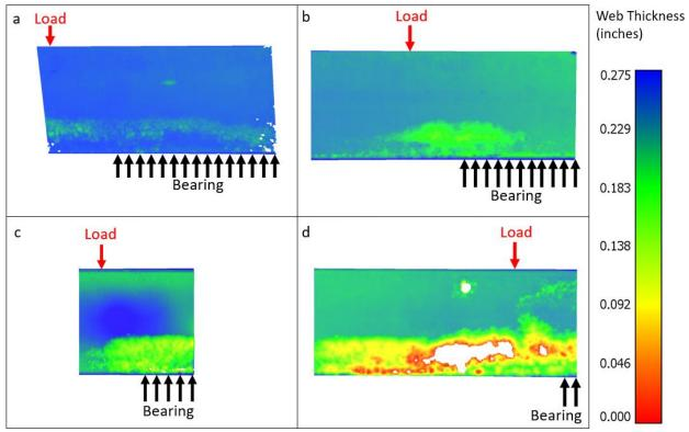
Figure 25. Heat Maps Showing Web Thickness of W10x26 Beam End Specimens: (a) 5-W10-L; (b) 6-W10-ML; (c) 7-W10-MH; (d) 8-W10-H.
