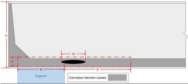
Figure 45. Critical Dimensions Used for Load Rating Corroded Steel Beams
