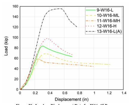
Figure 30. Load vs. Displacement Data for W16x45 Beams
