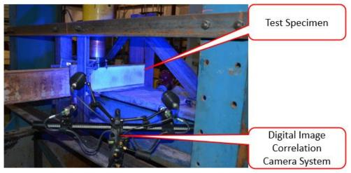
Figure 10. Digital Image Correlation Camera Scanning a Beam
