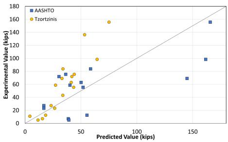
Figure 43. Prediction Error Plot for AASHTO and Tzortzinis et al. Capacity Calculations Using Remaining Average Thickness Over Corroded Web Portion
