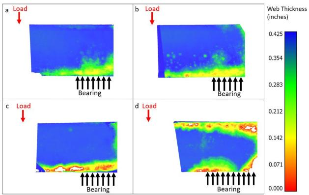
Figure 27. Heat Maps Showing Web Thickness of W21x62 Beam End Specimens: (a) 14-W21-L; (b) 15-W21-ML; (c) 16-W21-MH; (d) 17-W21-H.
