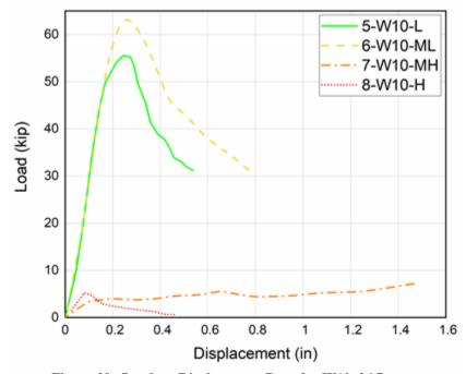
Figure 29. Load vs. Displacement Data for W10x26 Beams
