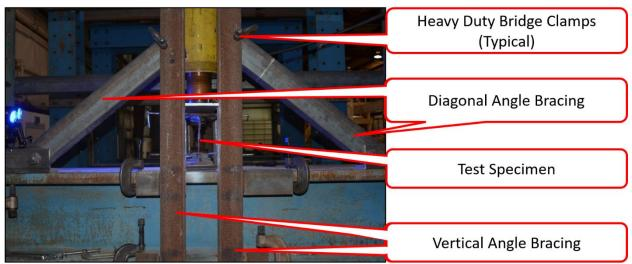
Figure 7. Beam End Bracing Configuration
