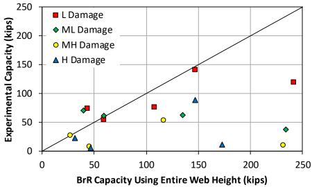
Figure 46. Comparison of Experimental and BrR Capacity. L = low; ML = medium-low; MH = medium-low; H = high.
