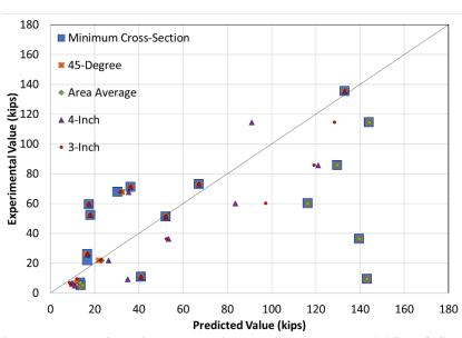
Figure 41. Prediction Error Plot of Maximum Experimental Shear Load vs. AASHTO Shear Capacity Using Five Thickness Measurement Methods
