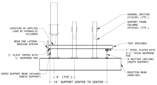
Figure 5. Elevation View of Full-Scale Beam Testing Configuration
