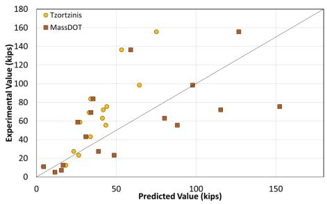
Figure 44. Prediction Error Plot for MassDOT and Tzortzinis et al. Capacity Calculation Methods
