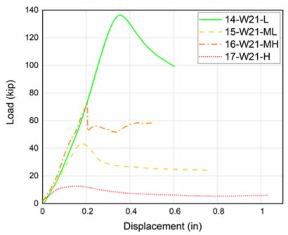
Figure 31. Load vs. Displacement Data for W21x62 Beams
