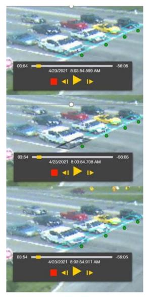
Figure 15. GS Software View of the Intersection Approach Showing Vehicles and Detection States
