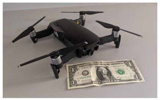
Figure 9. DJI Mavic Air<sup>®</sup> UAV of the Type Used for Aerial Video Collection at the Intersections
