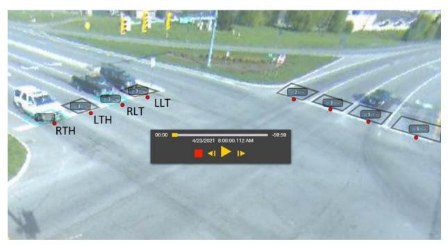
Figure 13. GS Camera View of SR 114 Eastbound and North Franklin Southbound Approaches Looking Northwest and Showing Vehicle Detection Zones, Viewing Tool Play Controller with Time and Lane Labels
