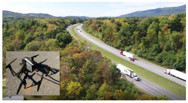
Figure 4. Video View Collected by the Tethered DJI Inspire 2 UAV (Inset) of I-81 Near Salem, VA
