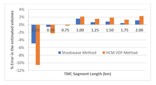
Figure 12. Average errors in estimating demand volume from the SW and VDF methods that are computed from the results of three simulation runs as TMC segment length is varied
