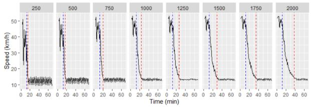
Figure 11. Speed profiles created from VISSIM data for different simulated TMC lengths ranging from 250 meters to 2000 meters (numbers shown at the top of each plot). The red dashed lines indicate t<sub>2</sub>, the times when the queue starts completely covering the TMC segment. The blue dashed lines indicate the times when the oversaturated period begins.
