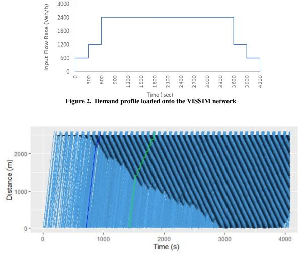
Figure 3. Vehicle trajectories for the simulated oversaturated condition. Two sample trajectories are highlighted (blue and green) for a better visualization.
