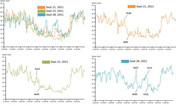
Figure 14. INRIX speed profiles for the XD segment on IRR over the three days
