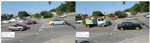
Figure 10. Sample images from the vehicle detection program
