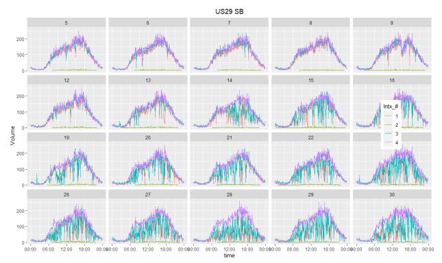
Figure 8. Five-minute volume profiles for the SB movements of four intersections on US 29 extracted from the ATSPM data for weekdays in April 2021. Numbers above the plots refers to the day of the month in April 2021. The names of the intersections can be found in the inset in Figure 7.
