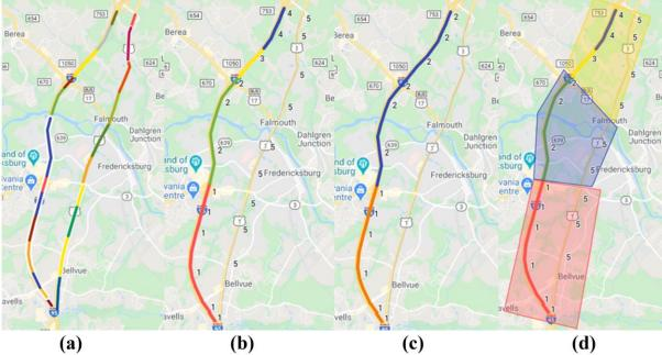
Figure 2. Example Illustrations of Spatial Segmentations Used in This Study: (a) INRIX XD segments; (b) links (constrained by adjacent interchanges); (c) corridors (unconstrained by adjacent interchanges); (d) sections (that include one or more interstate links and parallel arterial link[s]).
