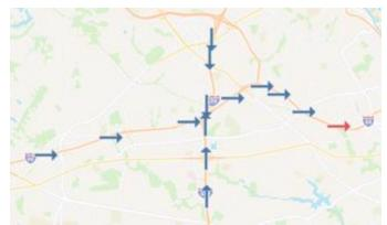
Figure 4. Illustration of Upstream Links (on I-66 Eastbound, I-495 Northbound, and I-495 Southbound in Blue) for a Given Link (on I-66 Eastbound in Red)
