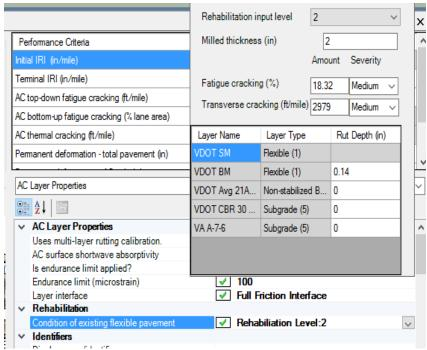
Figure A3. Level 2 Rehabilitation Input in Pavement ME Design
