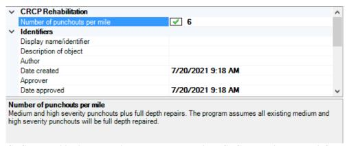
Figure A7. CRCP Rehabilitation Inputs in Pavement ME Design. CRCP = continuously reinforced concrete pavement.
