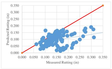
Figure 21. Comparison of Measured vs. Predicted Rutting for SMA Over JCP Projects. SMA = stone matrix asphalt; JCP = jointed concrete pavements.
