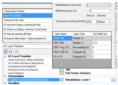
Figure A1. Level 1 Rehabilitation Input in Pavement ME Design
