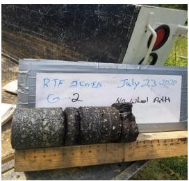
Figure 4. Core Showing Delamination in Multiple Layers and Moisture Damage at Bottom Layer (Rte. 250 EB, Richmond District)
