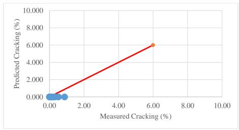
Figure 23. Comparison of Measured and Predicted Bottom-Up Cracking
