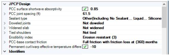
Figure A8. JCP Inputs in Pavement ME Design. JCP = jointed concrete pavement.
