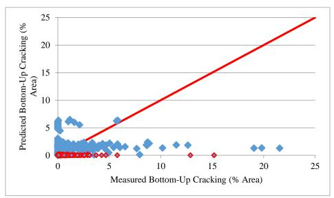
Figure 11. Comparison of Measured vs. Predicted Data. Data in blue are for new construction and are from a previous study (Smith and Nair, 2015); data in red are from the current study.
