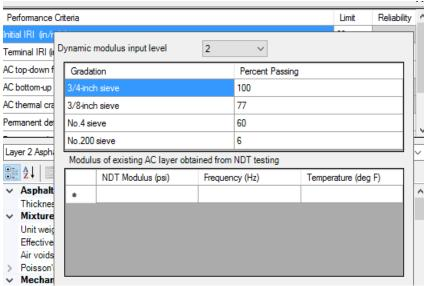
Figure A2. Level 1 Rehabilitation Input in Pavement ME Design (Backcalculated Modulus)
