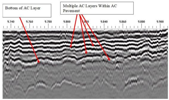
Figure 7. GPR Image of Rte. 250. GPR = ground penetrating radar.
