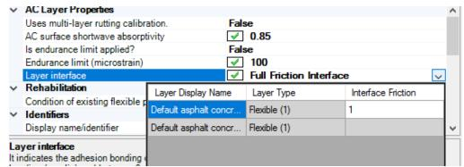
Figure A5. Example of Entering Interface Friction in Pavement ME Design
