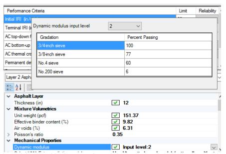
Figure A4. Rehabilitation Input for Existing Pavement in Pavement ME Design
