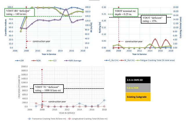
Figure A.2. Performance Plots and Structure for the SR40 FDR Emulsion Asphalt Project (Franklin County)
