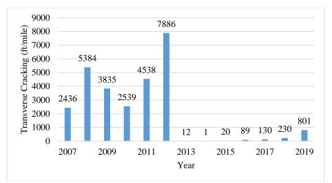
Figure 21. Transverse Cracking Data for Rte. 24. Full depth reclamation was completed in 2012 (after the 2012 condition survey).
