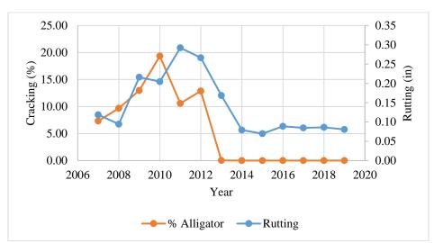
Figure 20. Rutting and Cracking Data for Rte. 24. Full depth reclamation was completed in 2012 (after the 2012 condition survey).
