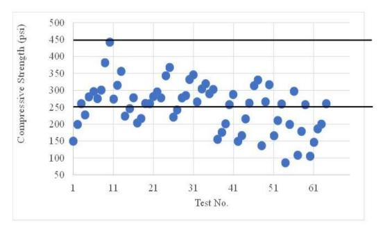
Figure 6. Compressive Strength Results for FDR Samples on Rte. 602. Horizontal lines indicate minimum and maximum acceptable values. FDR = full depth reclamation.
