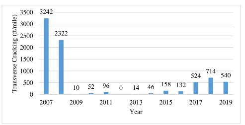
Figure 18. Transverse Cracking Data for Rte. 40 EB. Full depth reclamation was completed in 2008 (after the 2008 condition survey).
