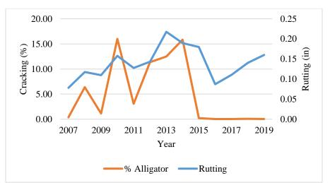
Figure 23. Rutting and Cracking Data for Rte. 30. Full depth reclamation was completed in 2014 (after the 2014 condition survey).
