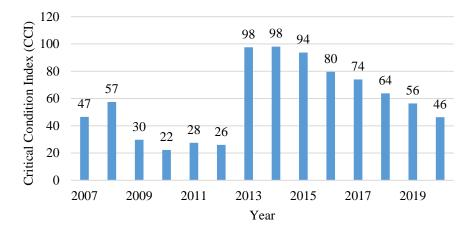
Figure 25. CCI Data for Rte. 3. Full depth reclamation was completed in 2012 (after the 2012 condition survey).
