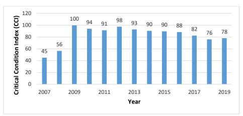
Figure 16. CCI Data for Rte. 40 EB. Full depth reclamation was completed in 2008 (after the 2008 condition survey).
