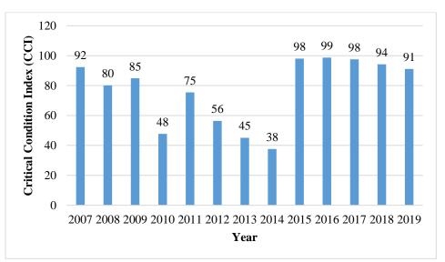
Figure 22. CCI Data for Rte. 30. Full depth reclamation was completed in 2014 (after the 2014 condition survey).
