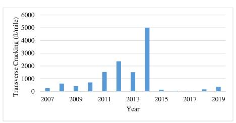
Figure 24. Transverse Cracking Data for Rte. 30. Full depth reclamation was completed in 2014 (after the 2014 condition survey).
