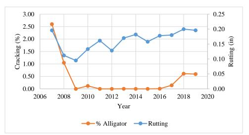
Figure 17. Rutting and Cracking Data for Rte. 40 EB. Full depth reclamation was completed in 2008 (after the 2008 condition survey).
