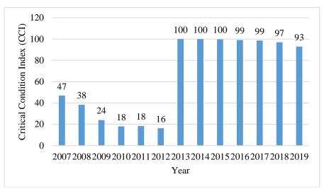
Figure 19. CCI Data for Rte. 24. Full depth reclamation was completed in 2012 (after the 2012 condition survey).
