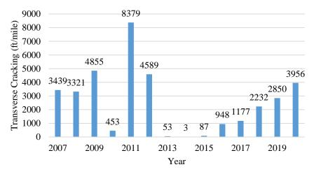
Figure 27. Transverse Cracking Data for Rte. 3. Full depth reclamation was completed in 2012 (after the 2012 condition survey).
