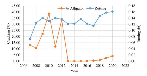
Figure 26. Rutting and Cracking Data for Rte. 3. Full depth reclamation was completed in 2012 (after the 2012 condition survey).
