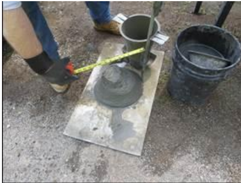
Figure 12. Slump Test for Batch 5
