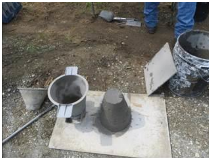
Figure 11. Slump Test for Stiff Batch 3
