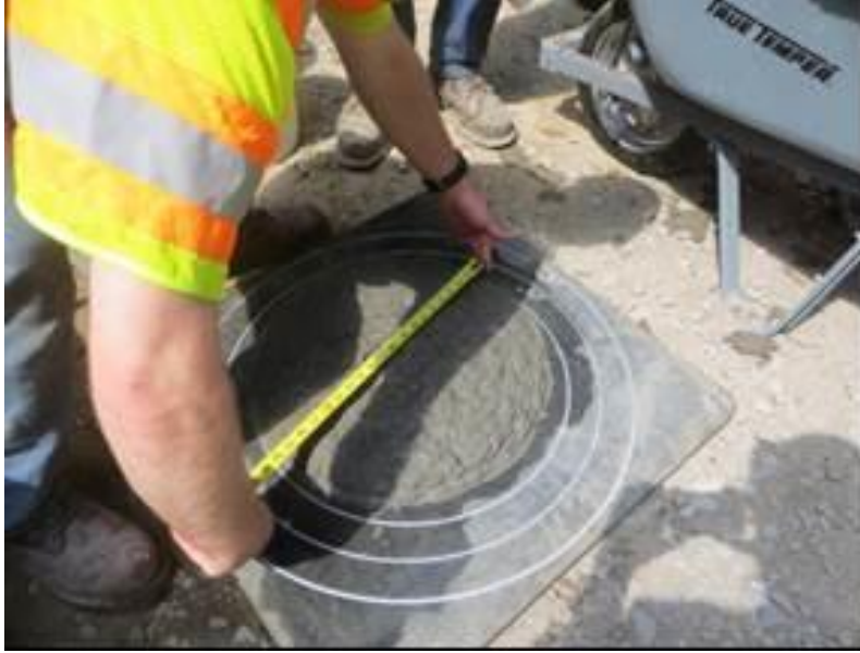
Figure 9. ECC in the Trial Batch and Mortar Mixer Batch. Batches 1 and 2 were self-consolidating, as shown by the measured slump flow. ECC = engineered cementitious composite.
