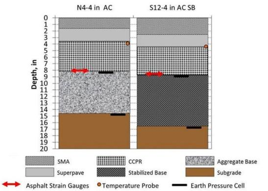
Figure 5. VDOT Sections at NCAT Test Track Showing Average As-Built Thicknesses and Depth of Instrumentation. VDOT = Virginia Department of Transportation; NCAT = National Center for Asphalt Technology; AC = asphalt concrete; SB = stabilized base; SMA = stone matrix asphalt; CCPR = cold central plant recycling.
