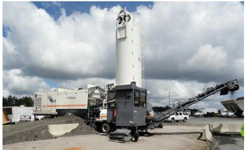
Figure 2. Mobile Plant Used for Cold Central Plant Recycling
