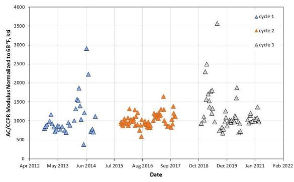
Figure 11. Section S12 Temperature-Normalized AC/CCPR Modulus. AC = asphalt concrete; CCPR = cold central plant recycling.
