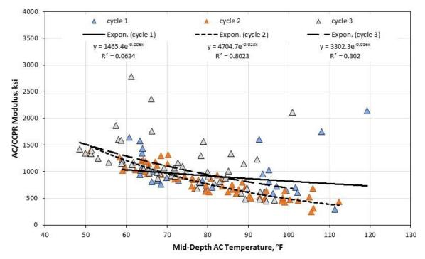
Figure 10. Section S12 AC/CCPR Modulus. AC = asphalt concrete; CCPR = cold central plant recycling; Expon. = exponential trendline.
