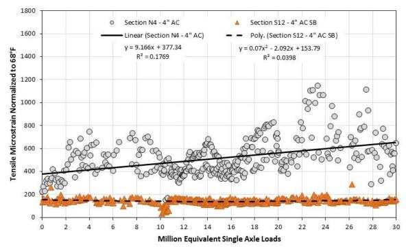
Figure 14. Horizontal Strain vs. Million Equivalent Single Axle Loads. AC = asphalt concrete; Poly. = polynomial trendline; SB = stabilized base.
