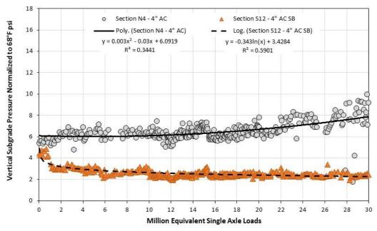
Figure 13. Vertical Subgrade Pressure vs. Million Equivalent Single Axle Loads. AC = asphalt concrete; Poly. = polynomial trendline; SB = stabilized base; Log. = logarithmic trendline.
