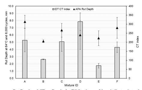
Figure 29. Average Rut Depth and  $CT_{index}$  Results for FC Specimens. I-bars indicate  $\pm 1$  standard deviation.
