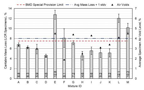
Figure 18. Average Cantabro Mass Loss and Air Voids for LCR Specimens. Average mass loss values are shown at the bottom of each column. I-bars indicate  $\pm 1$  standard deviation.
