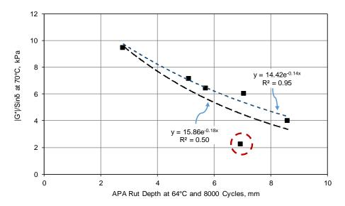
Figure 11. Correlations Between APA Rut Depth and  $|G^*|/\sin \delta$ . The circled data point appears to be an outlier.  $R^2$  improves from 0.50 (lower curve) to 0.95 (upper curve) when the circled point is removed from the analysis.
