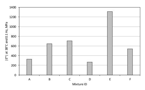
Figure 7. Dynamic Modulus |E\*| at 38°C and 0.1 Hz
