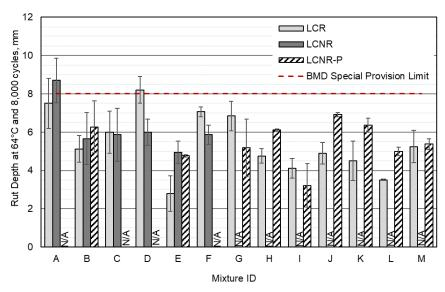
Figure 21. APA Rut Depths. Averages were computed from individual specimens tested in pairs. I-bars indicate  $\pm 1$  standard deviation.
