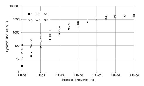
Figure 5. Dynamic Modulus |E\*| Master Curves
