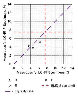
Figure 20. Effect of Multiple Operators Performing Specimen Fabrication on Mass Loss for LCNR vs. LCNR-P Specimens
