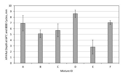
Figure 9. APA Test Results at  $64^{\circ}$ C and 8,000 cycles. I-bars indicate 1 standard deviation. APA = asphalt pavement analyzer.
