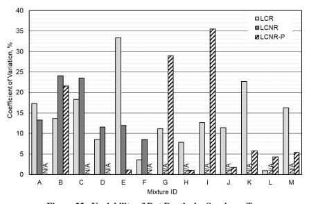
Figure 22. Variability of Rut Depths by Specimen Type
