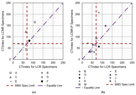
Figure 28. Effect of Reheating on CT<sub>index</sub> Values: (a) LCR vs. LCNR specimens; (b) LCR vs. LCNR-P specimens
