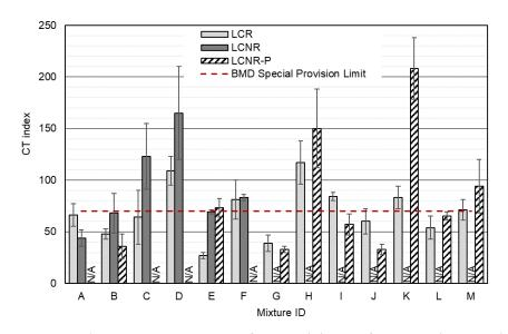
Figure 25.  $CT_{index}$  Results. Averages were computed from a minimum of three replicate specimens. I-bars indicate  $\pm 1$  standard deviation.
