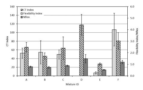
Figure 13. Cracking Test Results at 25°C
