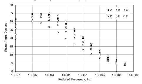
Figure 6. Phase Angle ( $\delta$ ) Master Curves
