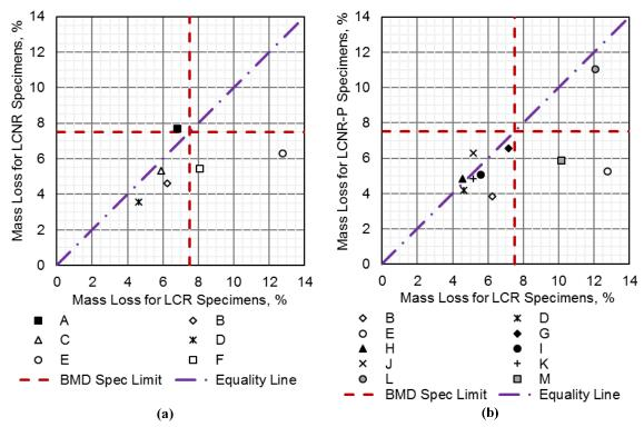
Figure 19. Effect of Reheating on Mass Loss: (a) LCR vs. LCNR Specimens; (b) LCR vs. LCNR-P Specimens
