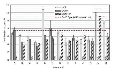
Figure 16. Cantabro Mass Loss Results. Values are the average of three replicates. I-bars indicate  $\pm 1$  standard deviation.
