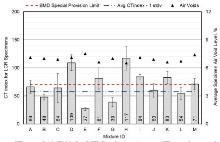
Figure 27. Average  $CT_{index}$  and Air Voids for LCR Specimens. Average  $CT_{index}$  values are shown at the bottom of each column. I-bars indicate  $\pm 1$  standard deviation.
