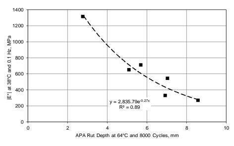
Figure 10. Correlation Between APA Rut Depth and |E\*| at 38°C and 0.1 Hz
