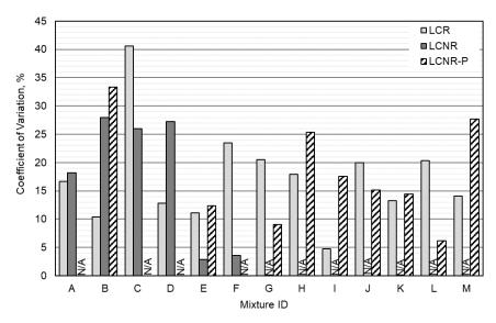
Figure 26. Variability of CT<sub>index</sub> Measurements by Specimen Type
