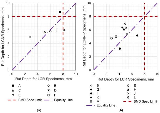
Figure 24. Effect of Reheating on Rut Depth Measurements: (a) LCR vs. LCNR specimens; (b) LCR vs. LCNR-P specimens
