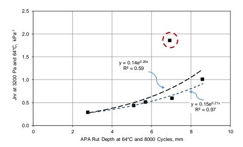
Figure 12. Correlations Between APA Rut Depth and  $J_{nr,3.2KPa}$ . The circled data point appears to be an outlier.  $R^2$  improves from 0.59 (upper curve) to 0.97 (lower curve) when the circled point is removed from the analysis.
