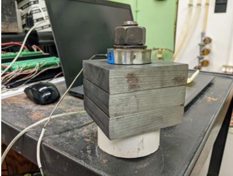
Figure 13. Photograph of Example 5-in-Long Bolt During Relaxation Test Sitting on Plastic Pipe
