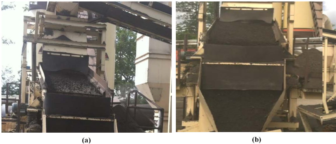
Figure 4. RAP Screen During Mixture Production: (a) 30% RAP; (b) 45% RAP. RAP = reclaimed asphalt pavement.
