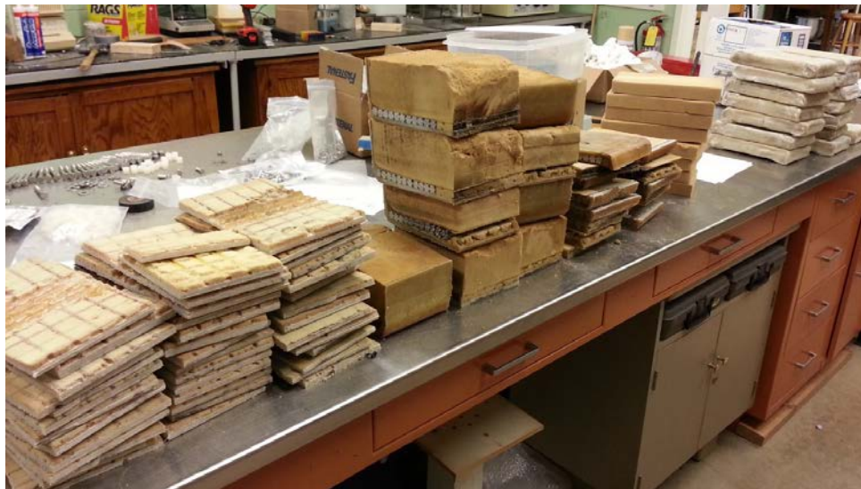
Figure 6. Hybrid Composite Beam Specimens Under Preparation
