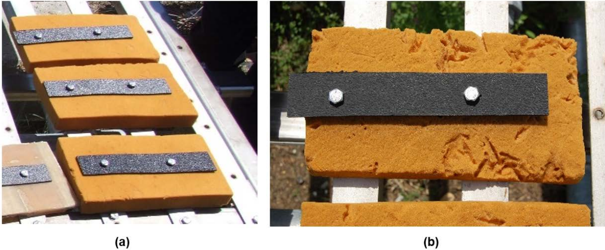
Figure 38. Comparisons of Foam Specimens: (a) initially; (b) after 1 year and 8 months showing how foam has degraded and exhibits loss of material, especially along the edge because of exposure
