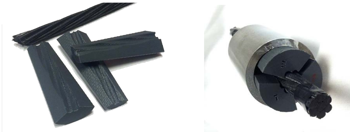
Figure 25. Anchor Wedges: (a) PEEK-G30; (b) 6061-T6 aluminum; (c) AISI 303 stainless steel.
