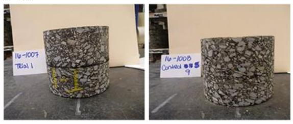
Figure 13. Cores from Route 611 Project: (left) from interlayer section; (right) from control section
