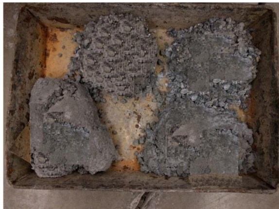
Figure 6. Concrete Mass Loss After Immersion. The two left samples had a slump of 7.75 in: the top left sample was from the basket; the bottom left sample was from the grout bag. The two right samples had a slump flow of 22 in: the top right sample was from the basket; the bottom left sample was from the grout bag.
