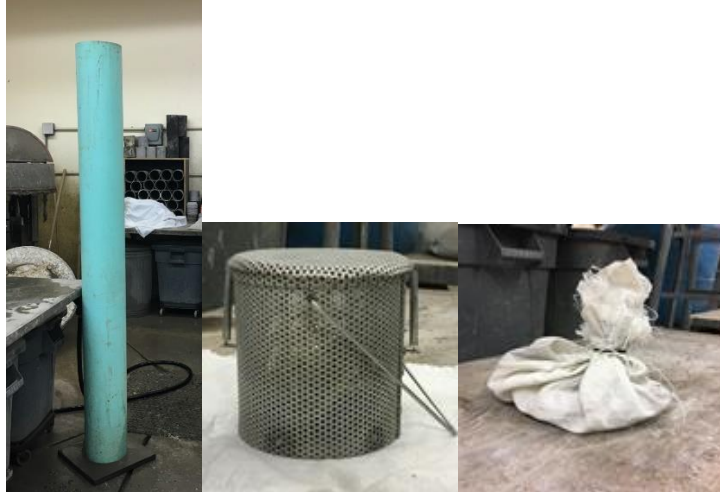
Figure 1. Underwater Column, Basket, and Grout Bag
