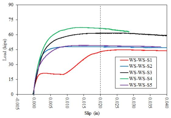
Figure A6. Plot of Compression Slip Test Data for WS-WS Specimens
