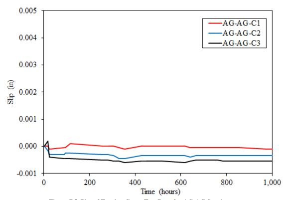
Figure B5. Plot of Tension Creep Test Data for AG-AG Specimens
