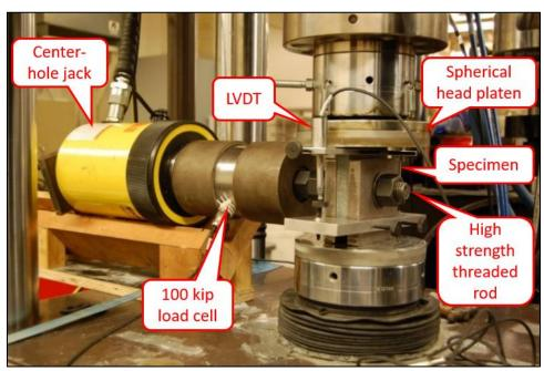
**Figure 4. Compression Test Setup**
