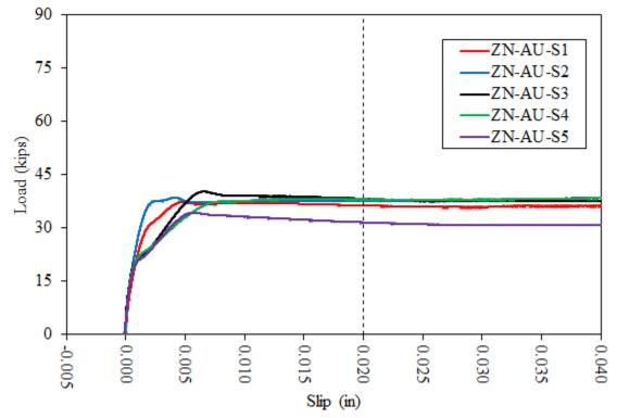
Figure 11. Plot of Compression Slip Test Data for ZN-AU Specimens
