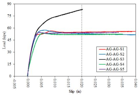
Figure 13. Plot of Compression Slip Test Data for AG-AG Specimens
