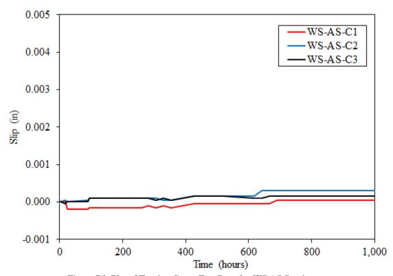
Figure B3. Plot of Tension Creep Test Data for WS-AS Specimens
