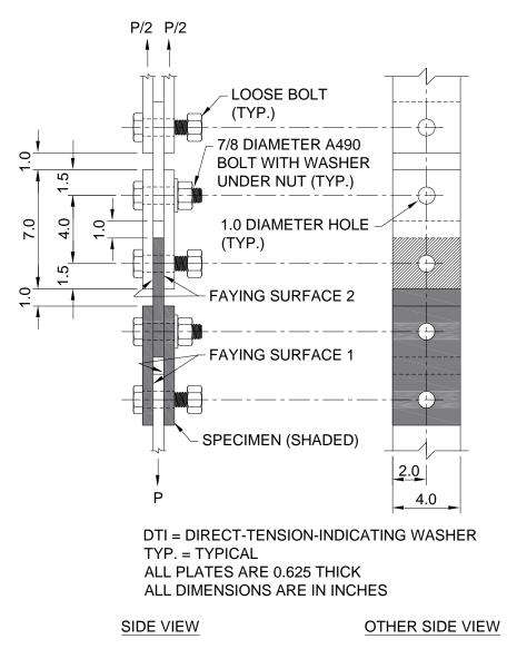
Figure 6. Drawing of Standard Tension Creep Test Specimens
