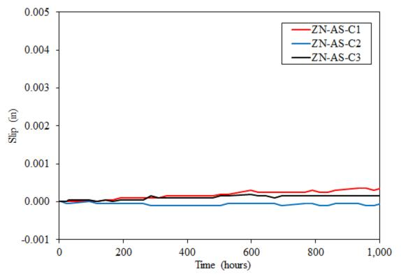
Figure B4. Plot of Tension Creep Test Data for ZN-AS Specimens
