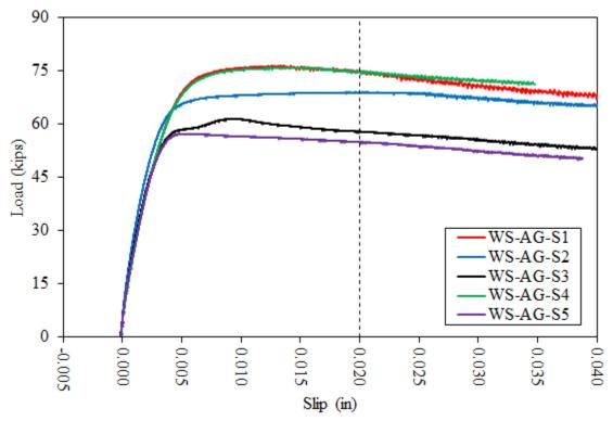
Figure A4. Plot of Compression Slip Test Data for WS-AG Specimens
