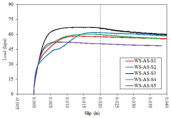
Figure A2. Plot of Compression Slip Test Data for WS-AS Specimens
