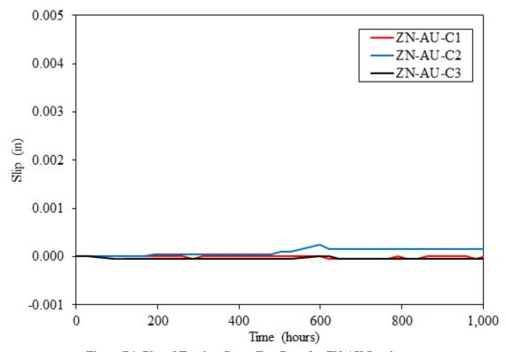
Figure B1. Plot of Tension Creep Test Data for ZN-AU Specimens
