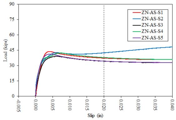
Figure A3. Plot of Compression Slip Test Data for ZN-AS Specimens
