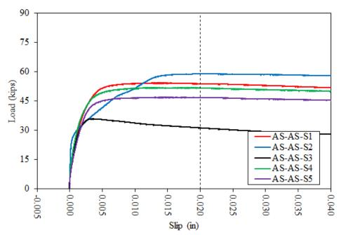
Figure 12. Plot of Compression Slip Test Data for AS-AS Specimens
