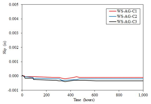
Figure B6. Plot of Tension Creep Test Data for WS-AG Specimens
