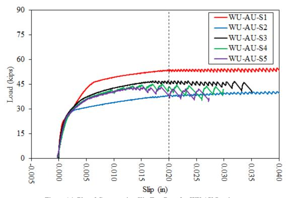
Figure A1. Plot of Compression Slip Test Data for WU-AU Specimens
