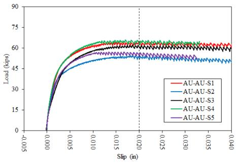
Figure 10. Plot of Compression Slip Test Data for AU-AU Specimens
