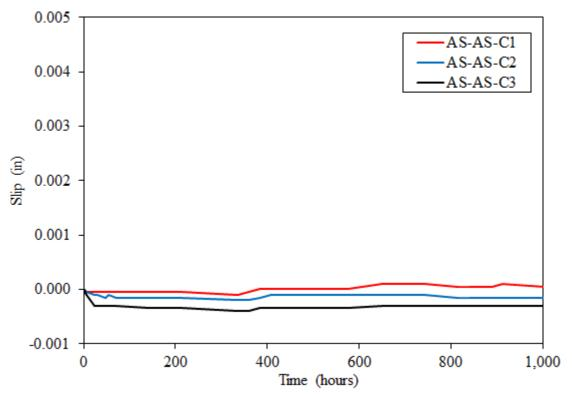
Figure B2. Plot of Tension Creep Test Data for AS-AS Specimens
