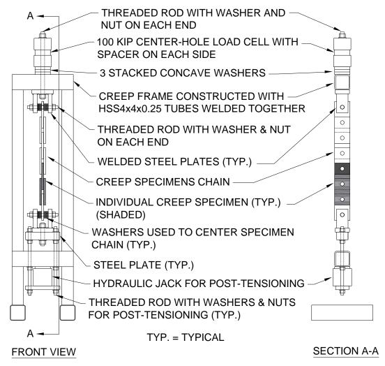
Figure 7. Drawing of Tension Creep Test Setup
