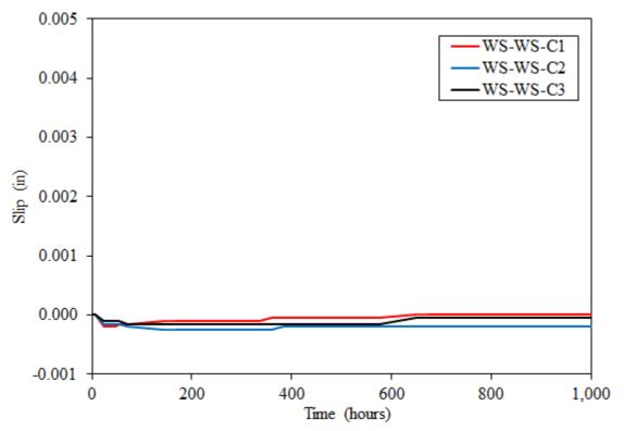
Figure B8. Plot of Tension Creep Test Data for WS-WS Specimens
