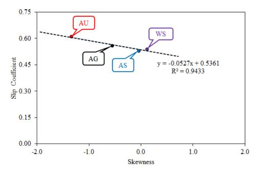
Figure 20. Plot of Experimental Slip Coefficient vs. Skewness of Height Data for Selected Faying Surface Types
