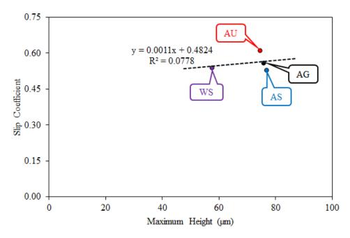
Figure 18. Plot of Experimental Slip Coefficient vs. Maximum Height for Selected Faying Surface Types
