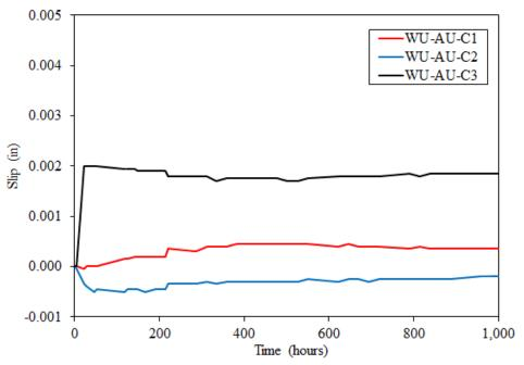
Figure 15. Plot of Tension Creep Test Data for WU-AU Specimens
