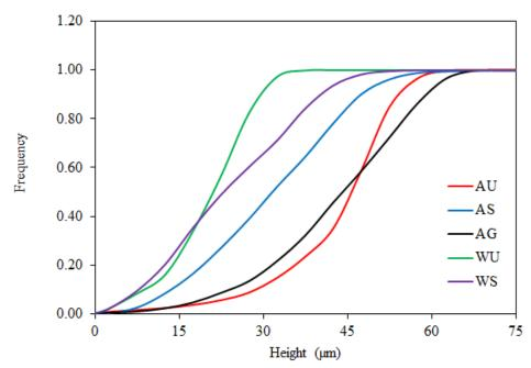
Figure 17. Cumulative Distribution Graphs of Height Data From Selected Faying Surfaces
