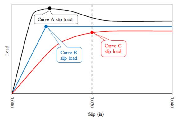
Figure 5. Definition of Slip Load
