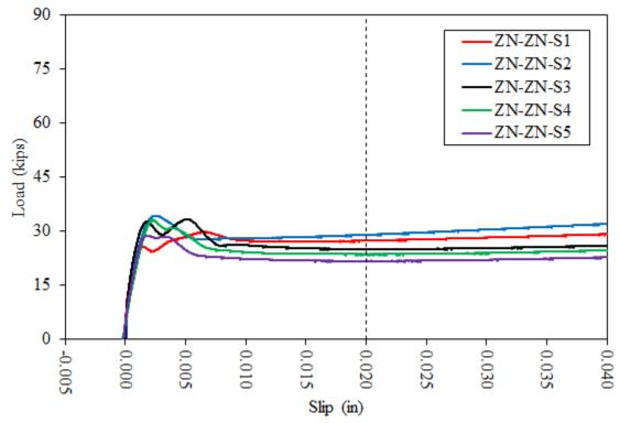
Figure A7. Plot of Compression Slip Test Data for ZN-ZN Specimens
