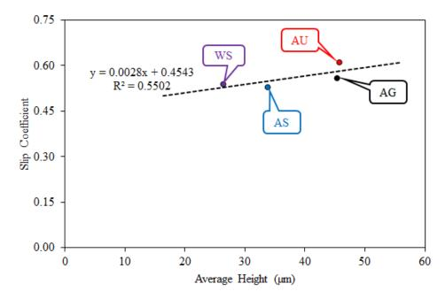
Figure 19. Plot of Experimental Slip Coefficient vs. Average Height for Selected Faying Surface Types
