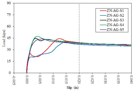
Figure A5. Plot of Compression Slip Test Data for ZN-AG Specimens
