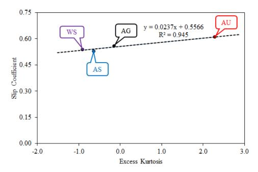
Figure 21. Plot of Experimental Slip Coefficient vs. Excess Kurtosis of Height Data for Selected Faying Surface Types
