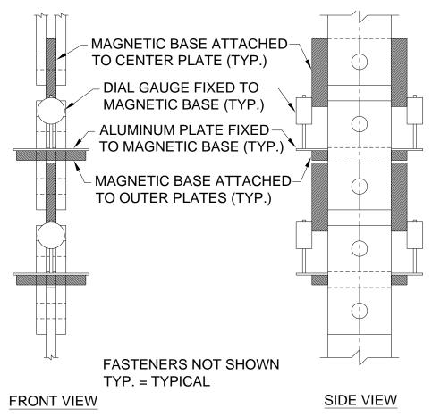
Figure 8. Drawing of Slip Measurement Instrumentation on Creep Test
