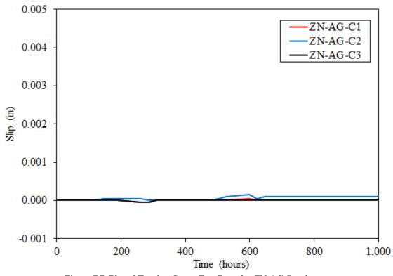
Figure B7. Plot of Tension Creep Test Data for ZN-AG Specimens
