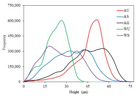
Figure 16. Line Histograms for Surface Profile Measurements of Selected Faying Surface Types
