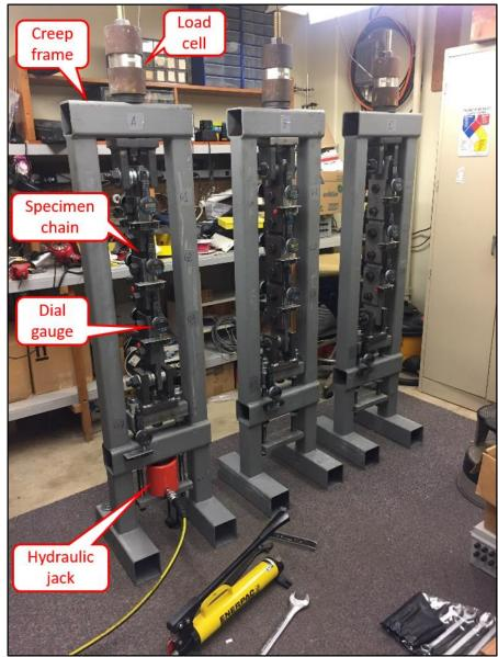
Figure 9. Photograph of Tension Creep Tests
