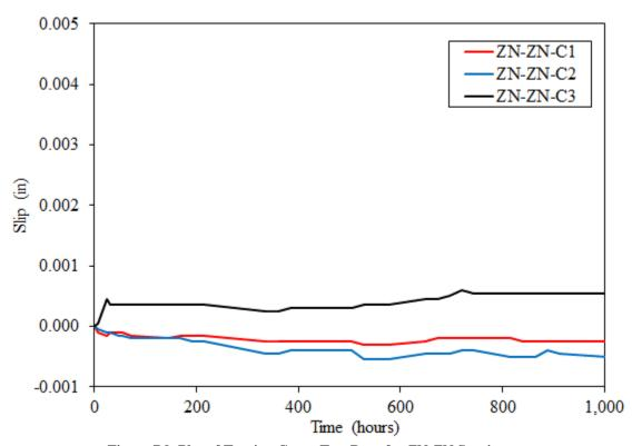
Figure B9. Plot of Tension Creep Test Data for ZN-ZN Specimens
