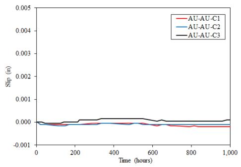
Figure 14. Plot of Tension Creep Test Data for AU-AU Specimens
