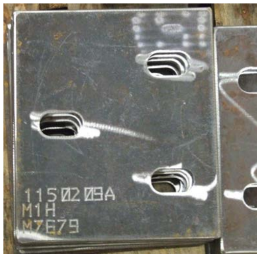
Figure 12. Identification Marking and Machining of A1010 Steel Plates Using Conventional Equipment
