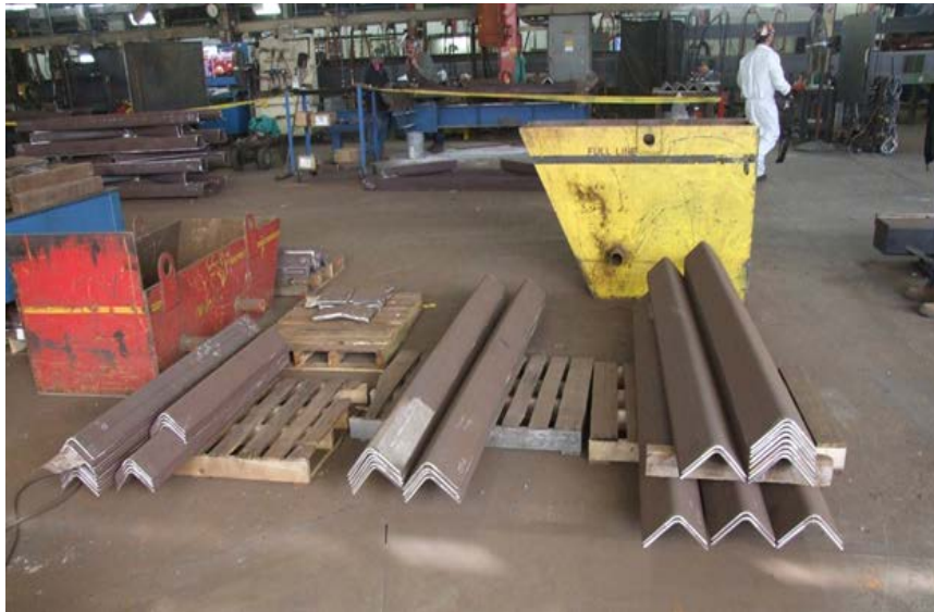
Figure 13. A1010 Steel Plate After Bending But Prior to Assembly
