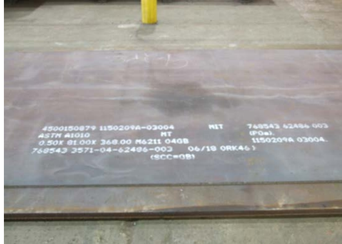
Figure 3. A1010 Steel Plate (½ in) Waiting to Be Moved to Cutting Table to Be Plasma Cut on Down Draft Table
