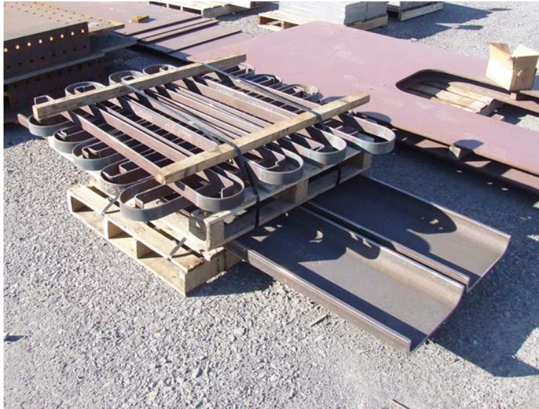
Figure 15. Water Line Support Brackets and Partially Fabricated Diaphragm After Bending
