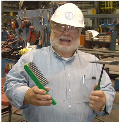
Figure 11. Hand Tools Marked With Green Paint to Indicate They Are Dedicated for Use on ASTM A1010 Steel Plate
