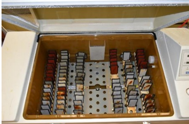
Figure 12. Coated Panels in Salt/Fog Chamber of Test Cabinet
