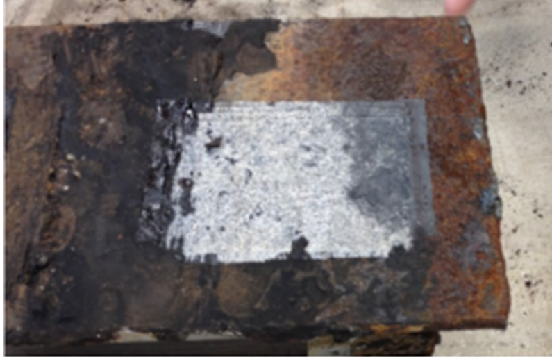
Figure 16. Laser-Cleaned Surface Area and Surrounding I-Beam Surface Area Prior to Cleaning
