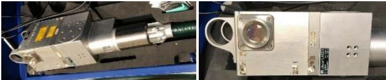
Figure 7. CleanCUBE H15 Optic Head Used With the 500 Watt Laser. The optical cable (green) enters the head from the laser power supply. The cleaning lens is on the left in both images.
