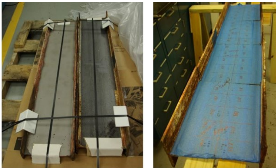
(a) (b) Figure 9. Steel Beams: (a) as received; (b) ready to be sawn into 3 in x 5 in panels
