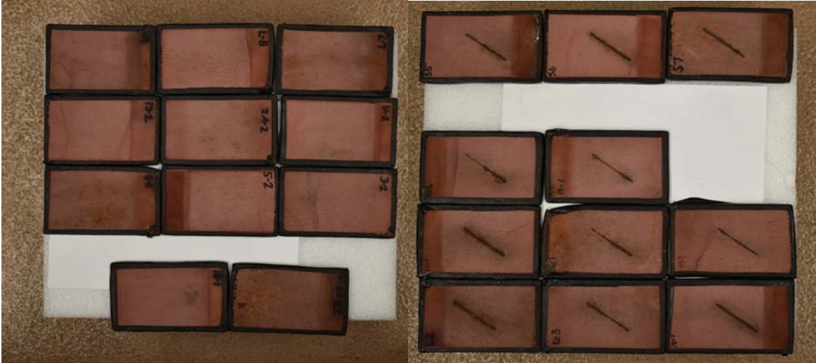
Figure 45. Panels Coated With Steel Spec Epoxy Primer. Grit-blasted panels are in upper row, and laser-ablated panels are in lower group.
