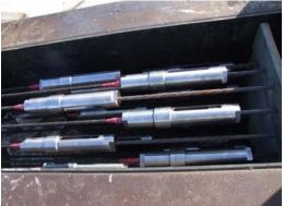
Figure 3. Elements of End Preparation: left, disassembled wedge, chuck, and braided grip; right, couplers in a pile
