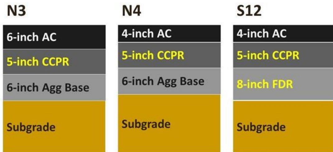
Figure 3. Schematic of NCAT Test Track Sections Including CCPR. The 8-in FDR layer was produced using an FDR process, but only unbound materials were reclaimed. The layer is called a “cement-stabilized foundation” in this report. NCAT = National Center for Asphalt Technology; CCPR = cold central plant recycling; FDR = full depth reclamation; AC = asphalt concrete; Agg = aggregate.
