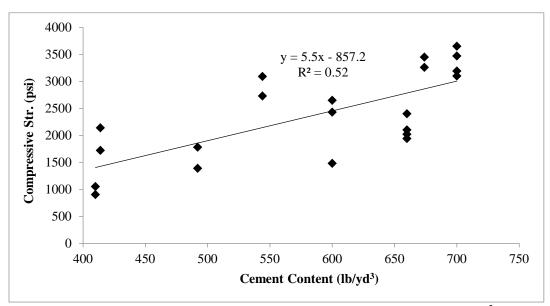
Figure 8. Compressive Strength (psi) As a Function of Cement Content (lb/yd<sup>3</sup>)
