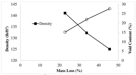
Figure 10. Density (lb/ft<sup>3</sup>) and Void Content (%) As a Function of Mass Loss (%)
