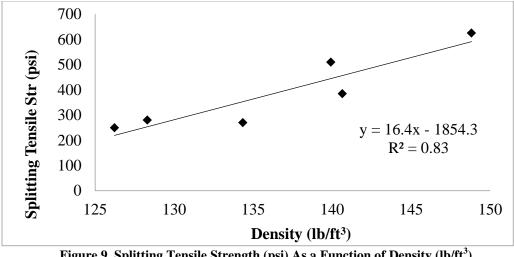
Figure 9. Splitting Tensile Strength (psi) As a Function of Density (lb/ft<sup>3</sup>)
