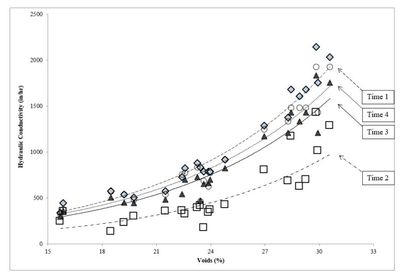
Figure 11. Hydraulic Conductivity (k) (in/hr) As a Function of Void Content (%): (1) Gray Diamonds: k Prior to Clogging Solution; (2) Squares: k After the Solution Containing Sand and Clay; (3) Triangles: k After One Vacuuming; (4) Circles: k After Both Pressure Washing and Vacuuming
