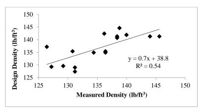
Figure 5. Design Density as a Function of Measured Density (lb/ft<sup>3</sup>)
