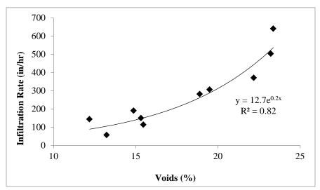
Figure 4. Results of ASTM C1701 Testing, Infiltration Rates (in/hr) Plotted Against Void Content (%)
