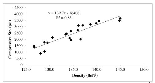
Figure 7. Compressive Strength (psi) As a Function of Density (lb/ft<sup>3</sup>)
