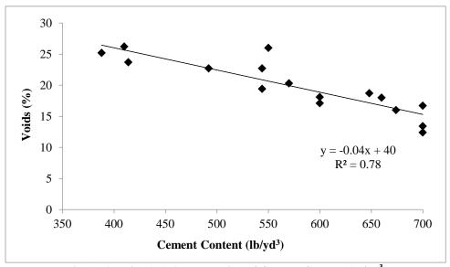
Figure 6. Voids (%) As a Function of Cement Content (lb/yd<sup>3</sup>)
