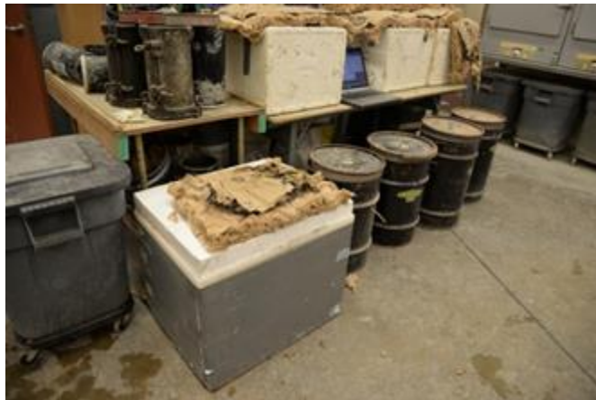
Figure 3. VES-FRCs Specimens Curing for First 24 Hours
