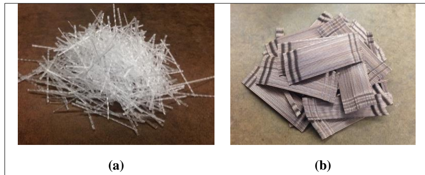
Figure 1. Fiber Types: (a) Polypropylene; (b) Steel
