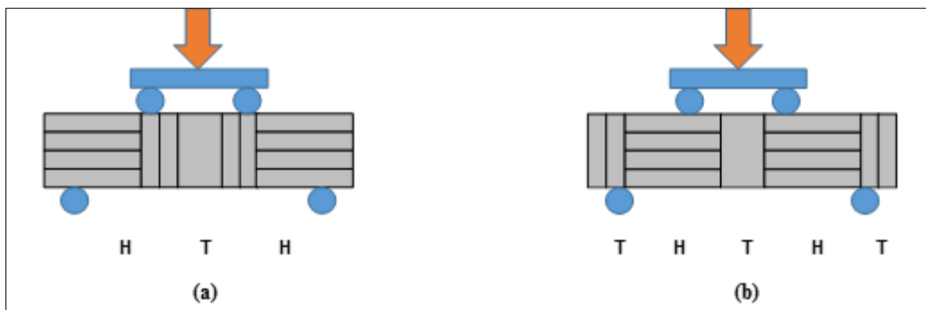
Figure 6. Schematic of Flexural Test Setup and Two Slicing Methods: (a) HTH, and (b) THTHT. H is a horizontal cut, and T is a transverse cut.
