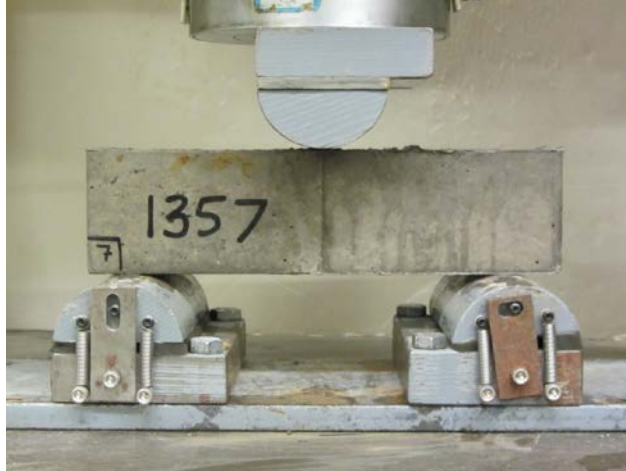
Figure 6. Setup for California Test 551
