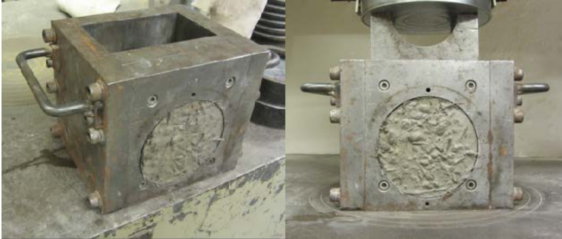
Figure 4. Setup for Guillotine Shear Test
