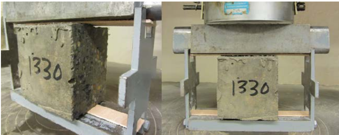
Figure 5. Setup for Splitting Prism Test. Note in left photograph that the base and high-performance fiber-reinforced concretes contain aggregate of several different colors and the interface plane is aligned with the axis of the slitting tensile loading head.
