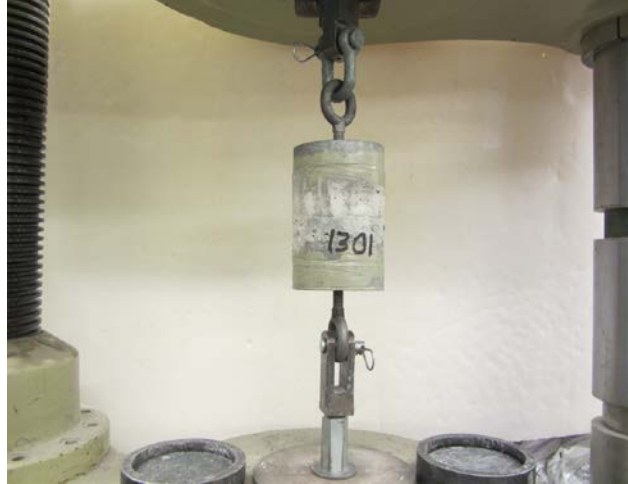
Figure 3. Setup for Direct Tension Bond Test
