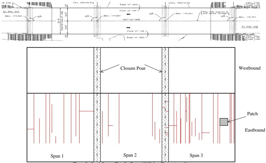
Figure 8. Crack Survey Plots for Route 646 Nokesville (not to scale)
