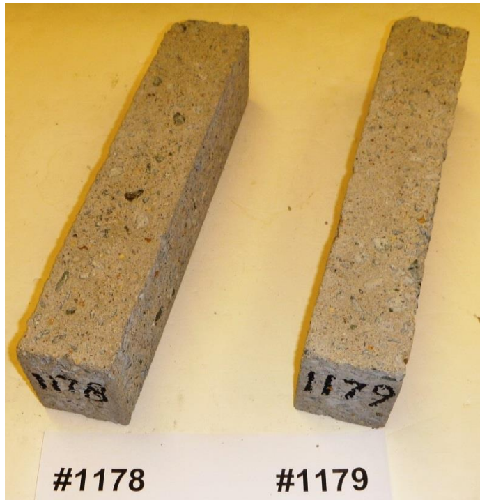
Figure 10. B607 Freeze-Thaw Beam Specimens After 300 Cycles
