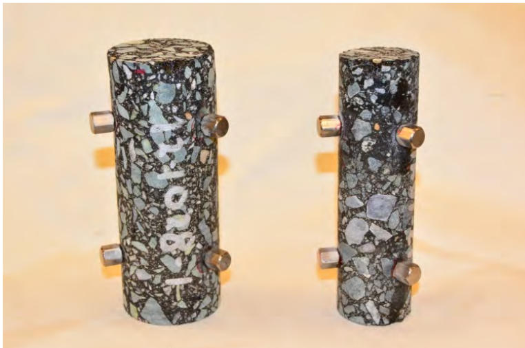
Figure 5. Examples of 38 mm ( right ) and 50 mm ( left ) in Diameter Small-Scale Cylindrical Specimens Prepared for Testing
