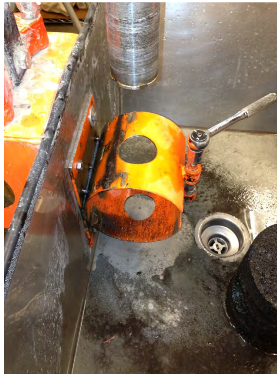
Figure 3. Core Drill Sample Holder Used to Extract Small-Scale Cylindrical Specimens From Gyratory Sample
