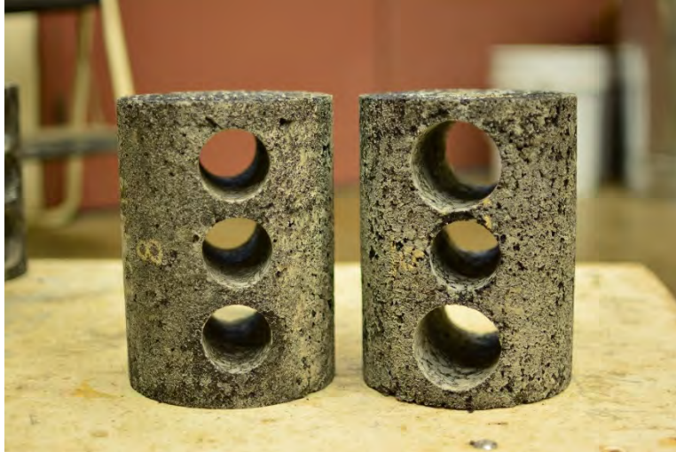
Figure 4. Gyratory Samples After Small-Scale Cylindrical Specimens Were Cored
