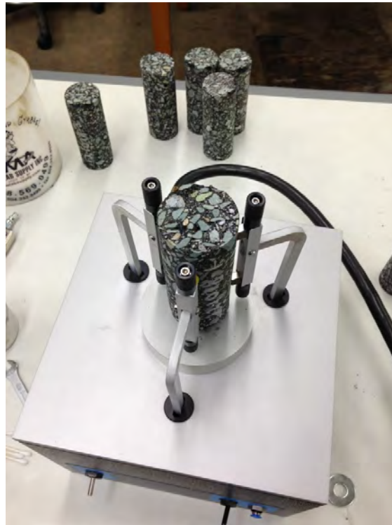
Figure 1. Photograph of LVDT Stud Gluing Jig Showing Custom Arms
