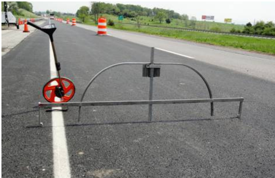
Figure 11. Six-Foot Rut Beam and Measurement Wheel Used During Manual Rut Depth Measurements
