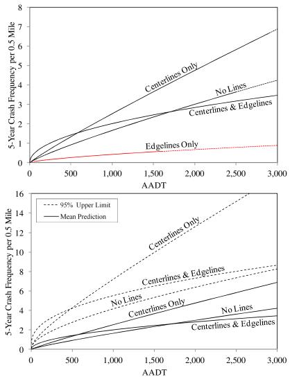
Figure 4. Safety Performance Function Results of 4 Segment Groups. *Top:* Mean Crash Predictions. The solid line indicates the range of actual AADTs, and the dotted lines indicate the range of AADTs that are not found in the data. *Bottom:* Mean Crash Predictions and 95% Confidence Limits.
