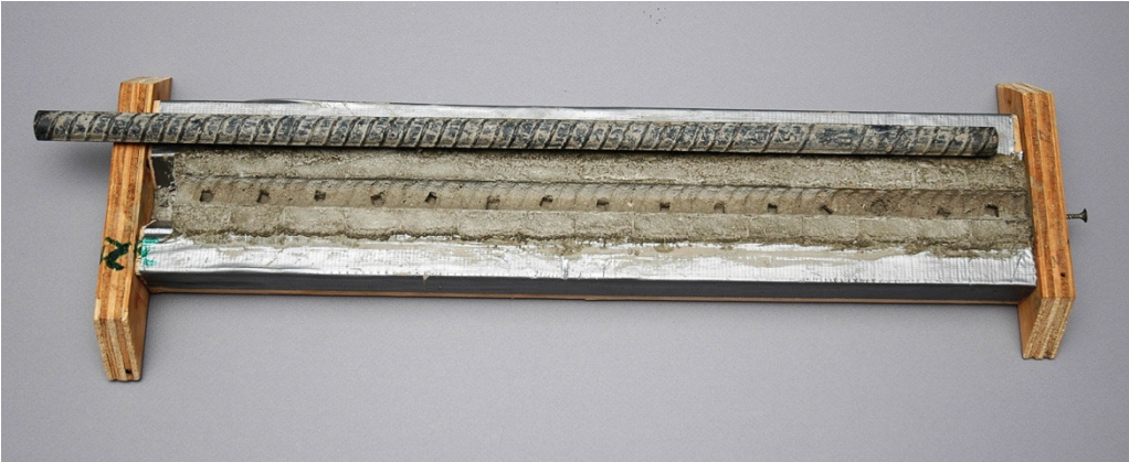
Figure 2. Wedges After Casting But Before Separation Into Individual Units
