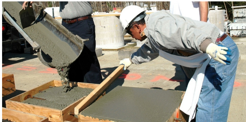
Figure 11. High Flow of SCC Makes Placement Work Easier. Concrete is placed in a second specimen without the need for vibrator while previous specimen is quickly screeded. SCC = self-consolidating concrete.
