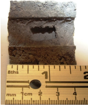
Figure 4. Single Wedge Before Placement Showing Larger Void (approximately 2 cm by 1 cm by 1 cm)
