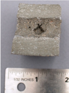
Figure 3. Single Wedge Before Placement Showing Small Void (approximately 1 cm by 1 cm by 1 cm)
