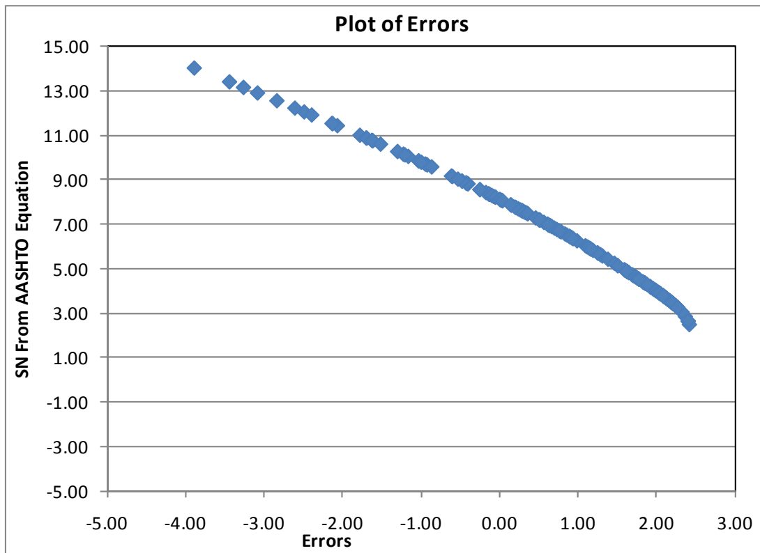
Figure 30. Plot of Errors: Closed Form Equation Minus AASHTO Equation
