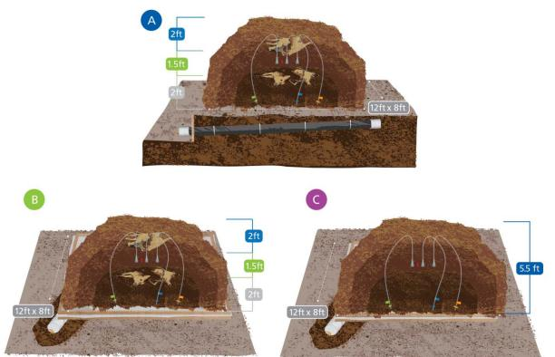
Figure 5. Illustrations of Plot Design, Windrow Construction, and Placement of Flasks Containing Pathogens: Windrow 1 (A), Windrow 2 (B), and control pile (C). A data logger was placed between the pathogen flasks in all three piles.
