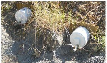
Figure 3. Plot 1: Drainage valves at lower end of lysimeters.
