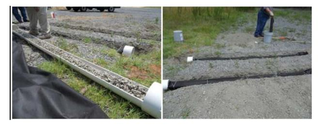
Figure 2. Plot 1: Lysimeters filled with aggregate (*left*), covered with landscaping cloth, and positioned 10 in beneath the soil surface (*right*).
