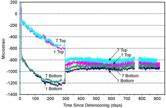
Figure 8. Strain Data for Span I Exterior Beams of Mattaponi Bridge
