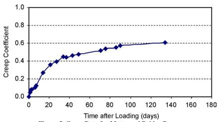
Figure 5. Creep Data for Mattaponi Bridge Beams
