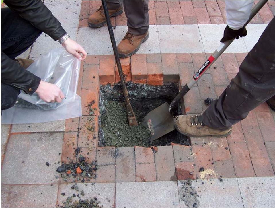
Figure B2. Specimen Collection of Aggregate Base at Intersection of 4th Street and High Street
