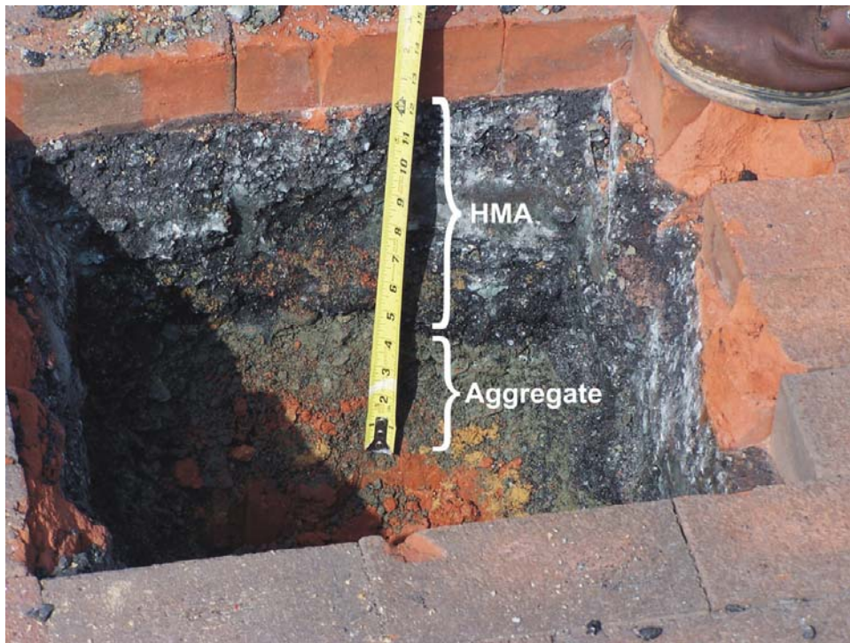
Figure B3. Measurement of HMA and 21-A Aggregate Base Layer at Intersection of 4th Street and High Street (approximately 7 and 5 inches, respectively)
