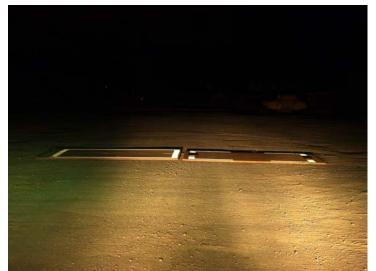
Figure 4. Outlined Plate and Corners Only Plate Under Low-Beam Headlights Zoomed in From 80 Feet
