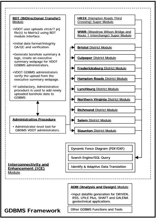
Figure 1. Schematic Relationship and Dependency Among Various GDBMS Framework Components
