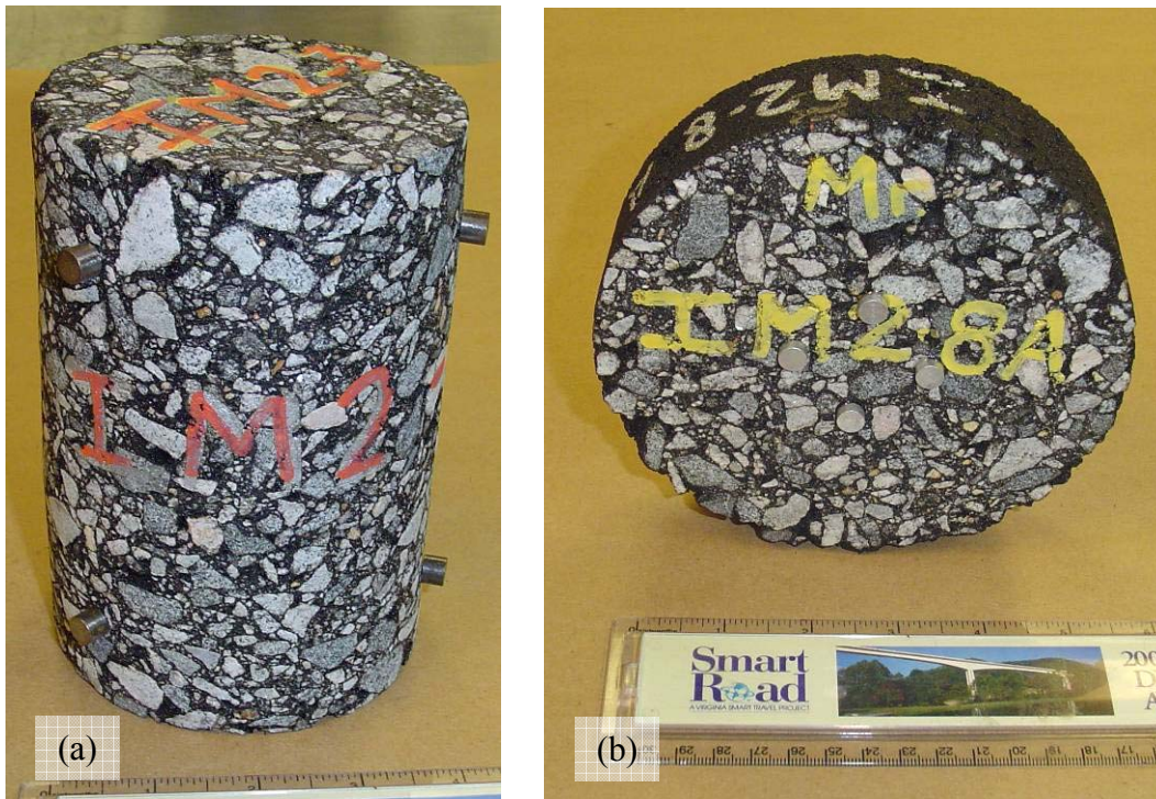
Figure 1. Typical specimens for (a) dynamic modulus and (b) resilient modulus and creep test
