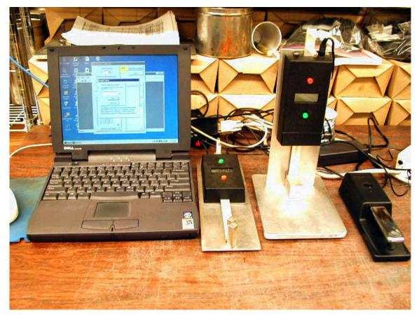
Figure 2. Digital Calipers. The horizontally operated caliper (HDC) with upright pins is in the center. The vertically operated caliper (VDC) with plates is the upright device near the right. The device on the far right is a foot (or elbow) pedal that permits the operator to initiate a reading when both hands are busy.
