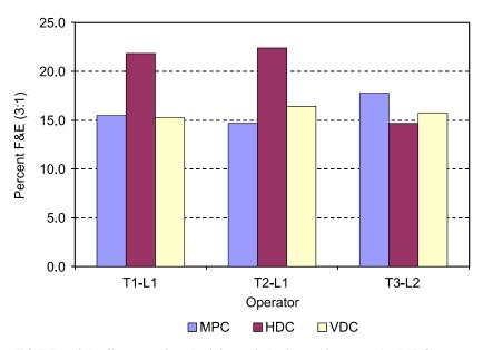
Figure 4. Average F&E Particle Content (3 technicians, 3 devices, 10 sources). MPC = manual proportional caliper; HDC = horizontal digital caliper; VDC = vertical digital caliper; T1-L1 = Technician 1-laboratory 1, etc.
