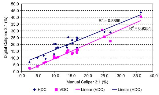
Figure 3. Digital Caliper Results as Function of Manual Caliper (Technician No. 1, 3 devices, 22 sources)
