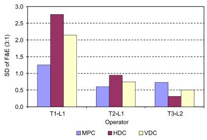
Figure 5. Average Standard Deviation of Measured F&E (3 technicians, 3 devices, 10 sources). MPC = manual proportional caliper; HDC = horizontal digital caliper; VDC = vertical digital caliper; T1-L1 = Technician 1-laboratory 1, etc.
